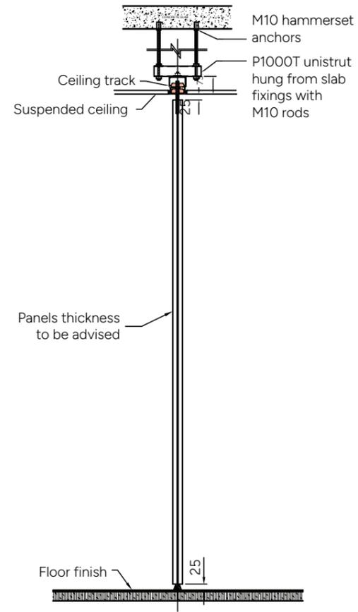
Vertical Section of Panel & Track Fixing
